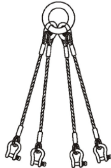
EEK 17 Four leg wire rope sling with main ring and intermediate ring at top with bow shackle at bottom.
