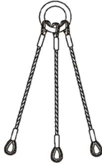
EEK 16 Three leg wire rope sling with main ring at top and thimble at the bottom.
